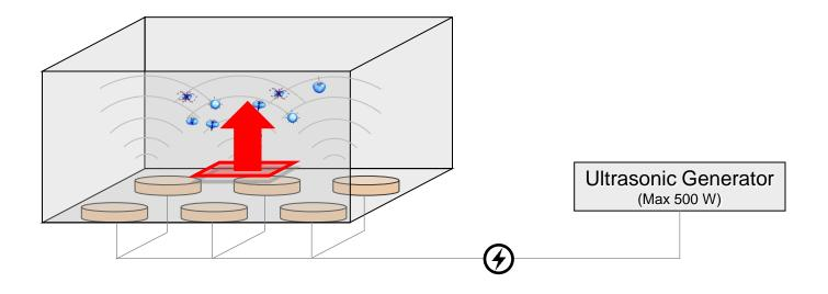
The same issues apply when measuring the Acoustic Intensity [W/cm<sup>2</sup>], which is defined by the acoustic power over a defined radiating area in the direction perpendicular to that area. It should be noted that the acoustic field is typically NOT uniform.
