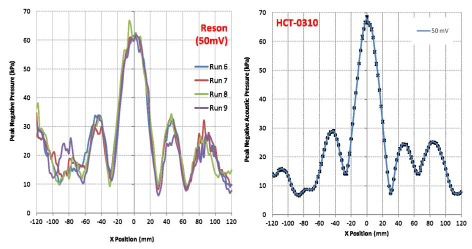
Good agreement seen between devices (similar dimensions and design), in field structure and measured pressure levels
